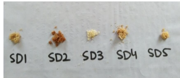
Figure 3: PHB crystals obtained by the bacterial isolates using sawdust as a low-cost substrate
