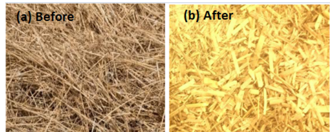
Figure 3: Wheat straw (a) Before and (b) After Physical Treatment [30]
