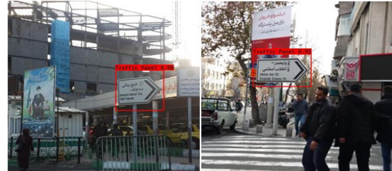
Figure 13: Instances of the correctly detected text-based traffic panels and other similar panels beside them.
