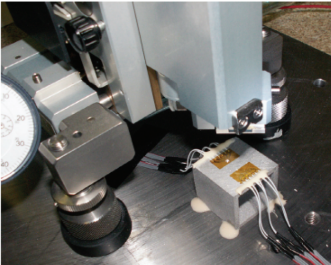
Figure 7: MTS3000 RESTAN (Residual Stress Analyzer) system [15].
