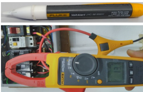
Figure 5: Comparing a current clamp meter with a volt detector
