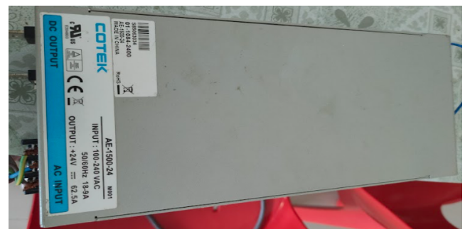
Figure 18: The SMPS used to power the electrically actuated valve.
