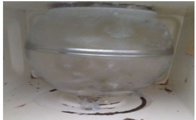
Figure 12: the glass container placed in the microwave oven and the top sealed with silicone
