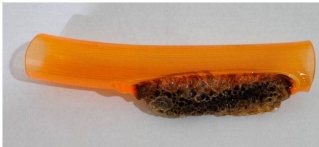
Figure 10: Plastic that melted in the microwave.
