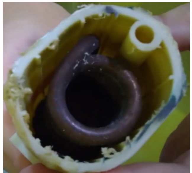
Figure 1: Some brands of heater element bathing heater use a plastic container where the water is heated up.
