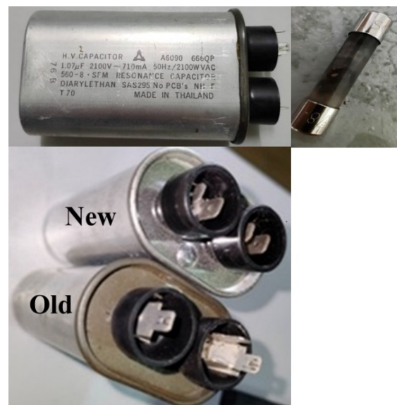
Figure 7: The top image is the capacitor that failed and the fuse that blew. The bottom image is the 1.07 \mu F, 2100 V capacitor that failed and its replacement.
