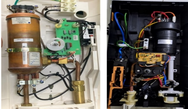
Figure 2: Some brands like Panasonic use a copper container to heat up the water and there is the green ground wire joined to this container. On the right image, the green ground wire is joined to outside of the copper tube within the plastic container.
