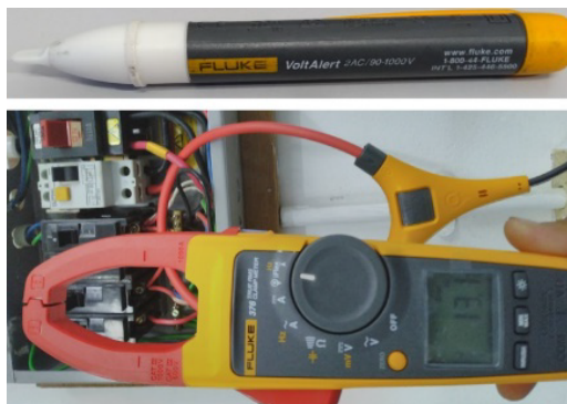
Figure 5: Comparing a current clamp meter with a volt detector
