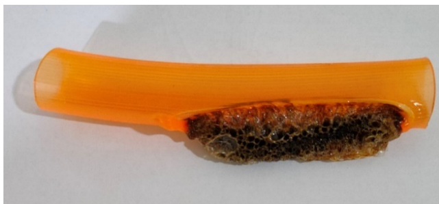
Figure 10: Plastic that melted in the microwave.
