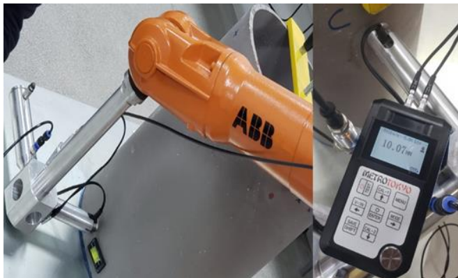
Figure 15: Example of automatic measurement performed by the robot in an unprecedented way with the value shown on the display.
