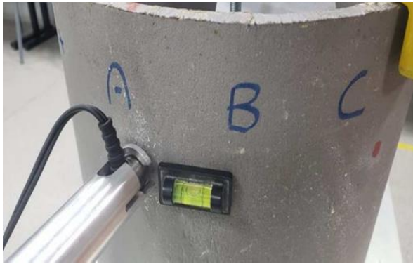
Figure 12: The ABC mesh on one side (right) of the pipe and the DEF mesh on the other side (left) of the pipe, together total 180 degrees of automatic measurement with the robot, divided into 10 layers with 40 distinct points.
