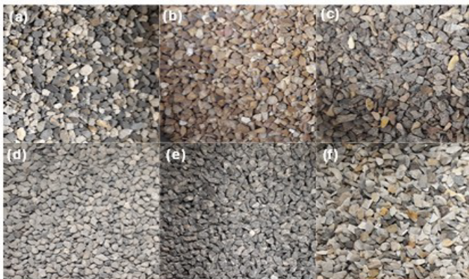
Figure 1: Calcined Bauxite and Alternatives: (a) Calcined Bauxite; (b) Meramec River Aggregate; (c) Rhyolite; (d) Steel Slag; (e) Earthworks; (f) Flint Chat
