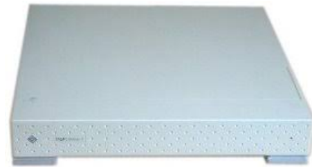
Figure 30: The “pizza box” containing the Sparcstation 1
