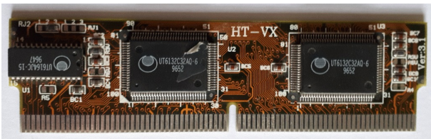
Figure 39: An example of an old cache module (DIMM).
