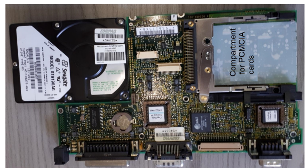
Figure 17: The other side of the card of Figure 16. Notice the PCMCIA card slot
