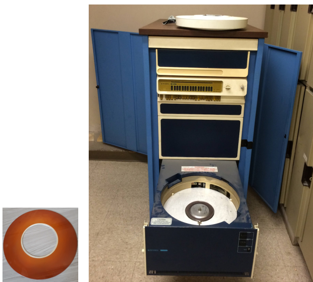
Figure 44: On the left, the plate of a Diablo disc; on the right, Data General's Nova 3 minicomputer equipped with a Diablo disk.
